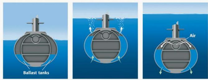
When a submarine is floating on the ocean's surface, its ballast tanks are filled mostly with air.
