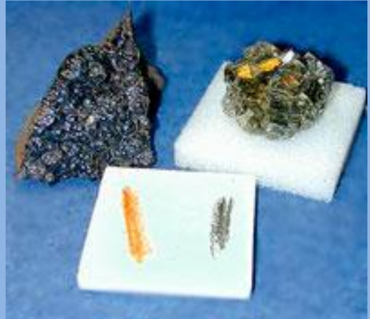
Streak plate test comparison of hematite and pyrite.
